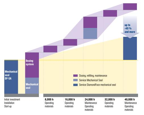
\* The calculation is based on a typical installation and operation of a feed water pump with mechanical seals with 140 mm (5.51") shaft diameter. The actual savings essentially depend on how the pump is operated. The statements made here indicate possible potentials through the use of mechanical seals with DiamondFace technology as compared to preceding installations at corresponding use and application. Video: DF-SA
